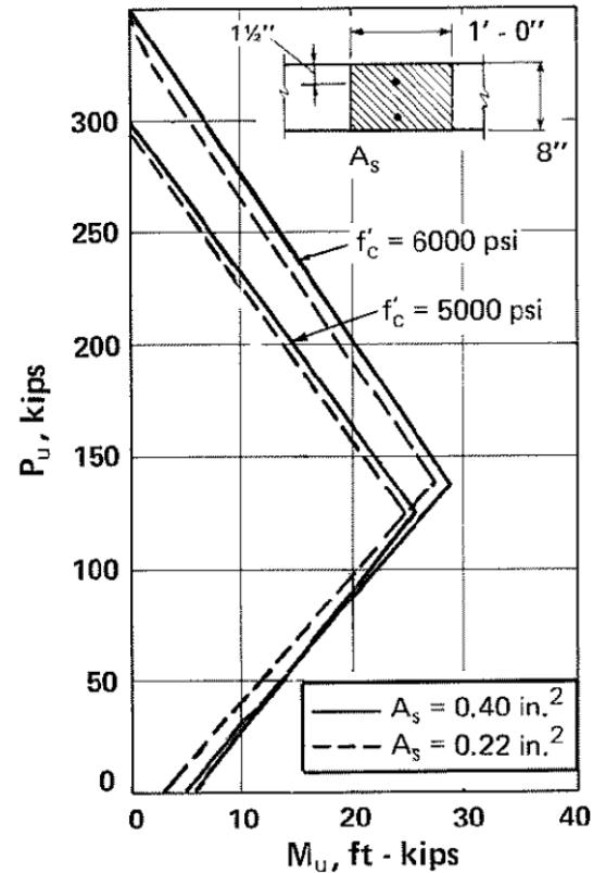
\*Curves based on an effective prestressing force in concrete of approx. 250 psi. Magnitude of prestress has negligible effect on capacity.
